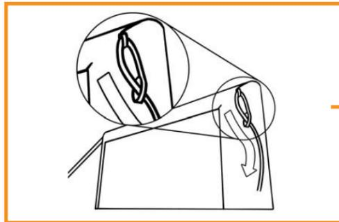
8. Secure all straps snug into the auger stakes. The eyelet will pull slightly-away from the unit which is a good sign that it is tight and secure.
